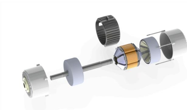
A typical NovaTorque motor design has a rotor/stator surface area interface that is twice the perpendicular cross-sectional area of the stator field pole. The increased surface area at the rotor/stator interface concentrates the magnetic flux density. This allows NovaTorque to use lower cost ferrite magnets to achieve motor efficiency and performance that equals or exceeds much more expensive motors that use rare-earth (neodymium) magnets.
